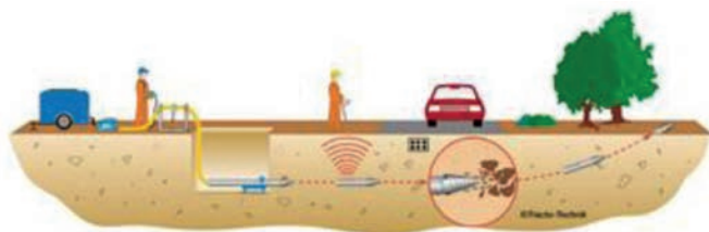
Rys. 6. Schemat metody GRUNDOSTEER Fig. 6. Schematic of GRUNDOSTEER method
