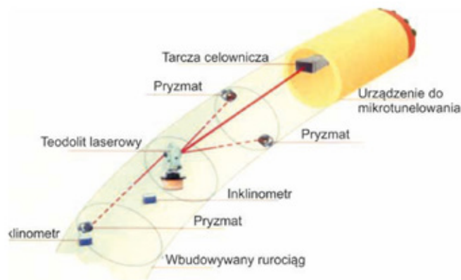
Rys. 8. Sterowanie procesem mikrotunelowania po łuku [10] Fig. 8. Controlling the microtunneling process along a curve
