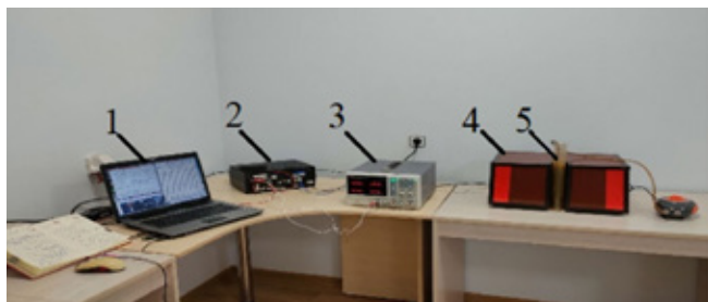
Fig. 3. A view of the installation for EMI activation of the ferritization process: 1 – computer; 2 – electronic block-case; 3 – power supply; 4 – electromagnetic coil with steel core; 5 – container with processed solution
