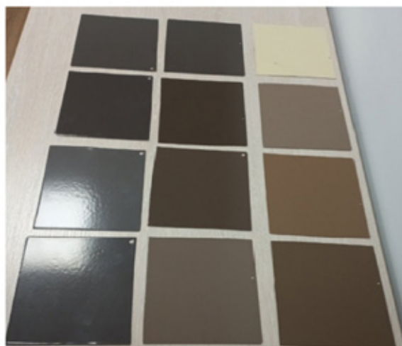
Fig. 5. Powder coatings with addition of 10 to 25% ferritization sediments from chromium-containing wastewater treatment.
