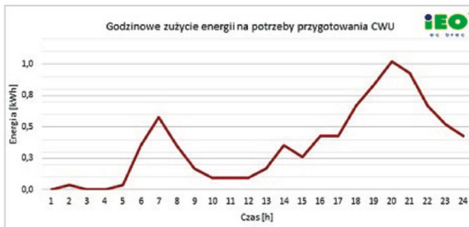
Fig.14. Hourly electricity consumption for hot water preparation [6]
