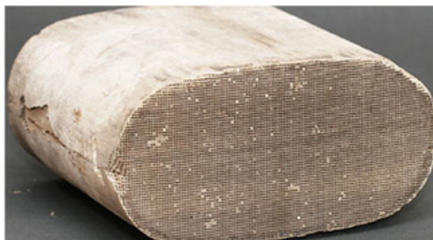
Fig. 1. View of spent auto catalysts on ceramic carrier
