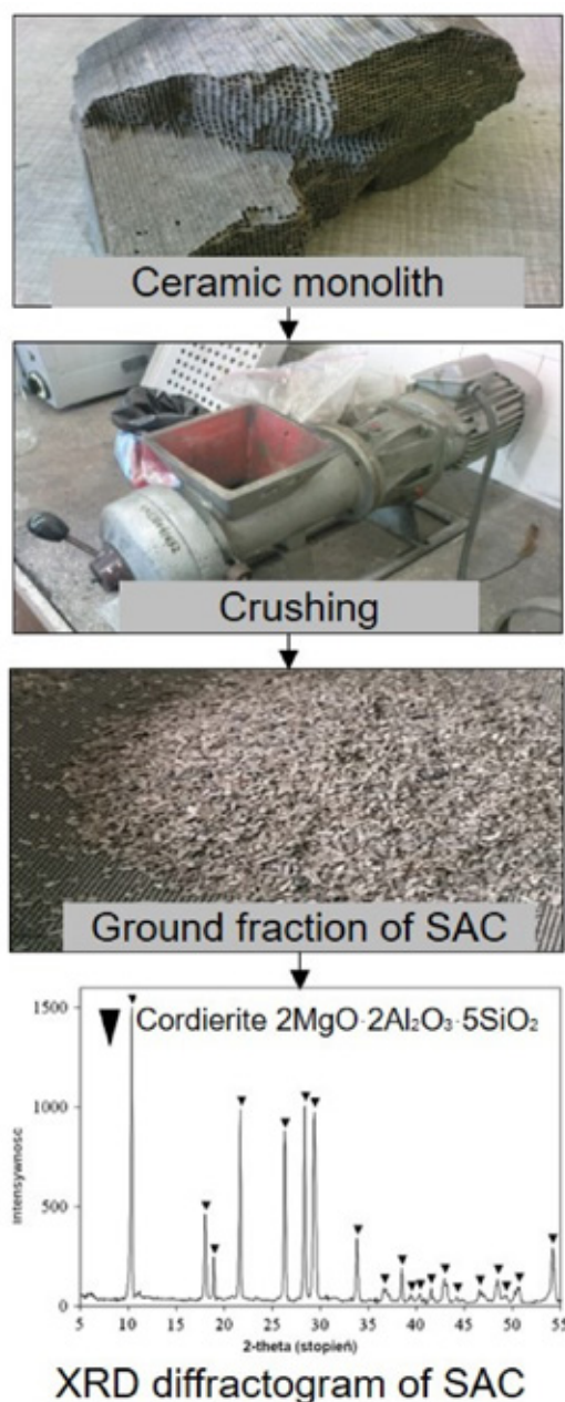
Fig.2. Scheme of the SAC cordierite material preparation process together with the sorption stage on the SAC bed
