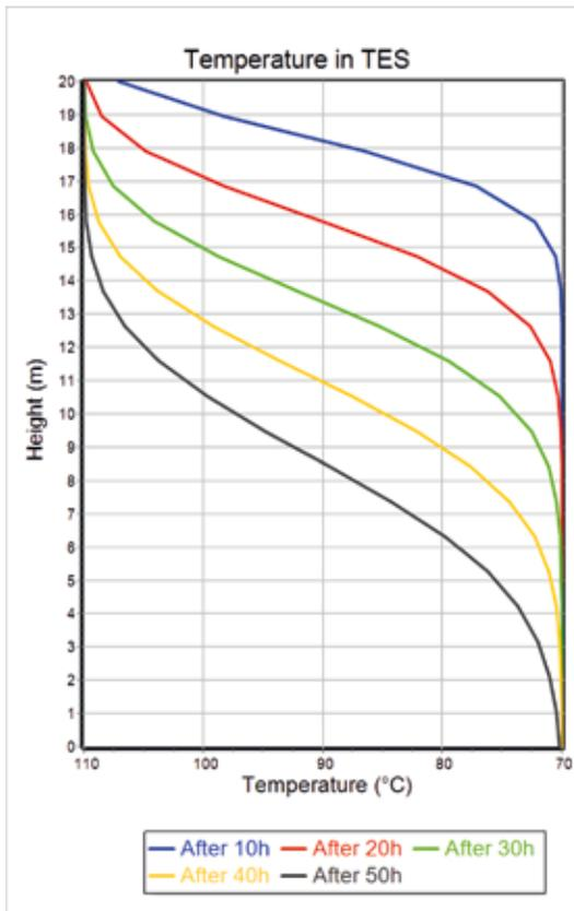
Fig. 2 Temperature change in TES for the balance equation
