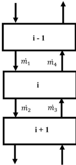
Fig. 1 Internal flows associated with node i
