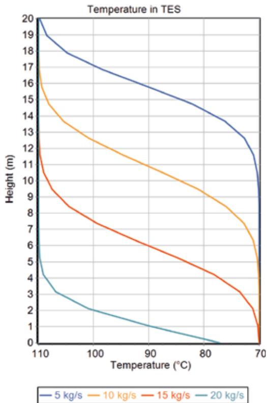
Fig. 8 Temperature change in TES for different charging flow rates
