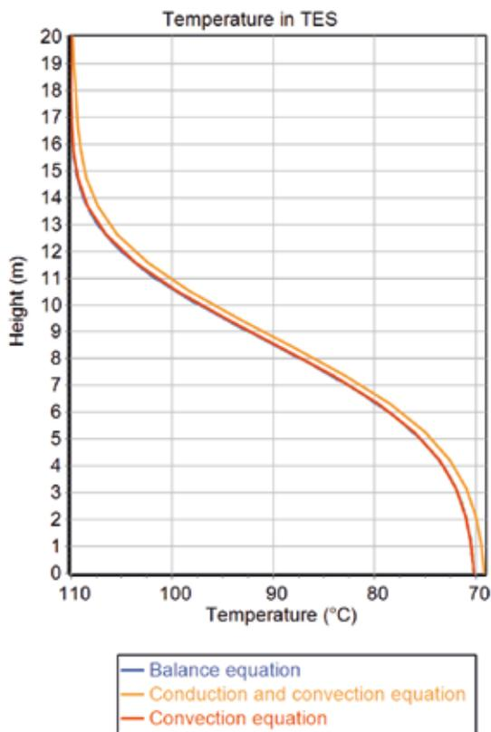
Fig. 5 Temperature change in TES for different equations (for 20 nodes)
