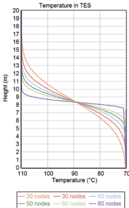
Fig. 7 Temperature change in TES for different nodes count
