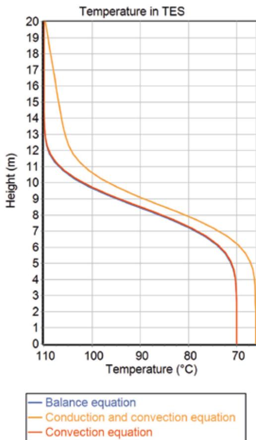
Fig. 6 Temperature change in TES for different equations (for 40 nodes)
