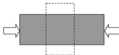
Fig.2: Contraction strain normal to the applied load
