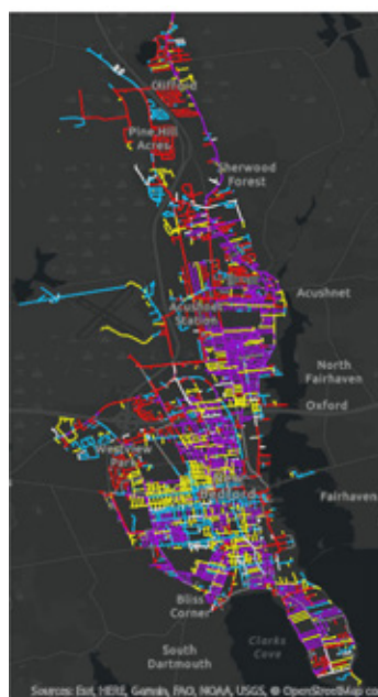
Fig.1. Compiled data over three drives (six passes) on each street showing vehicle breadcrumb (brown) and FOV coverage (blue)
