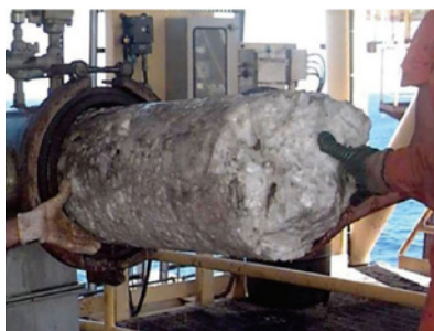
Fig. 3. Gas hydrate plug in a subsea pipeline [10].
