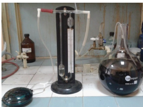
Fig. 2. Experimental unit for the study of the efficiency of biochemical aerobic treatment of the Chervonohrad MSW landfill filtrate
