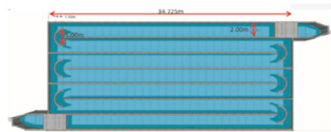
Fig. 8. Chlorination Tank and baffles
