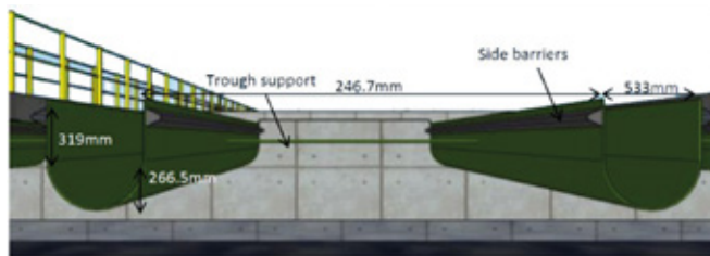
Fig. 3. Backwash troughs with dimensions
